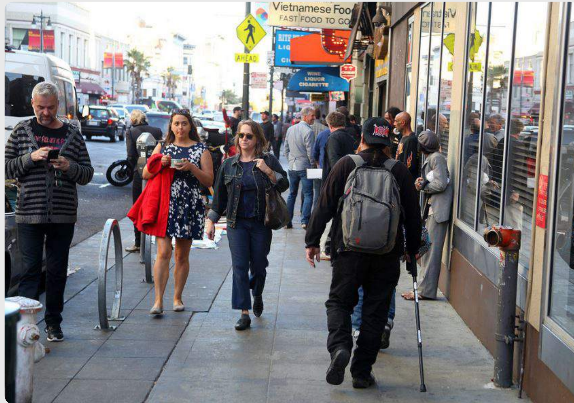
Narrow Sidewalks • 10' typical width 5' clear at pinch-points
