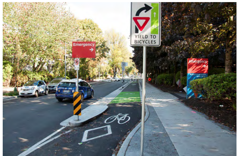
Figure 5: Protected Bike Lane in Vancouver, BC outside an Emergency Room provides horizontal and vertical deflection at the conflict point
