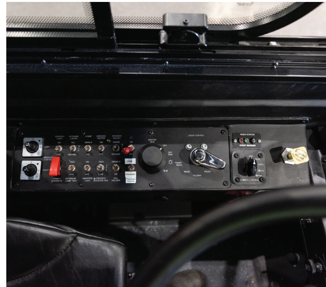
Figure 7-2: BYD bus 5004 Operator Side Panel Controls
