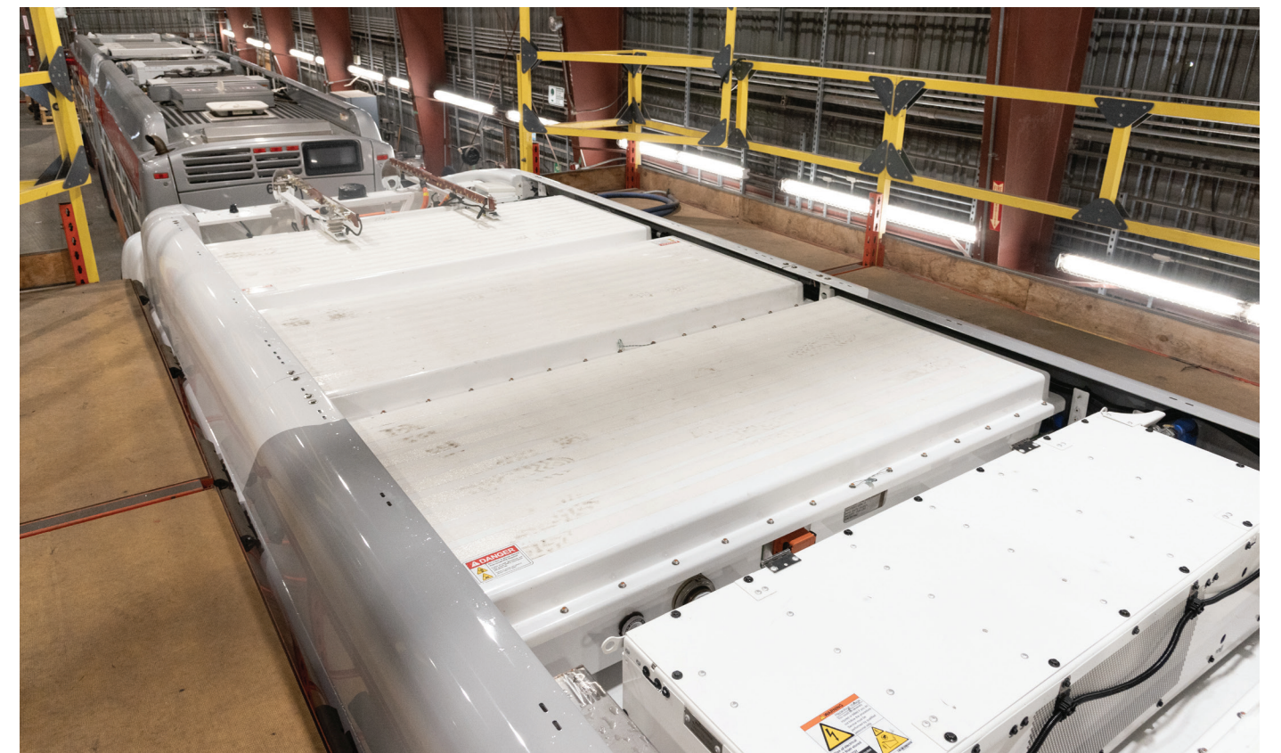
Figure 1-2: Rooftop Battery Units on the SFMTA's First Battery Electric Bus (New Flyer 5001)
