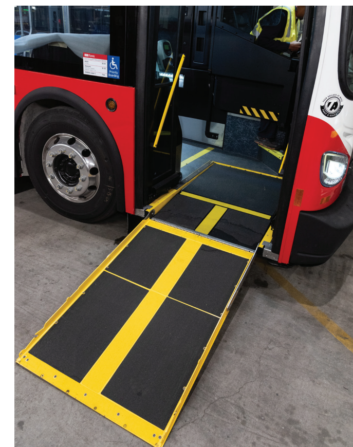
Figure 1-5: Upgraded Wheelchair Ramp
