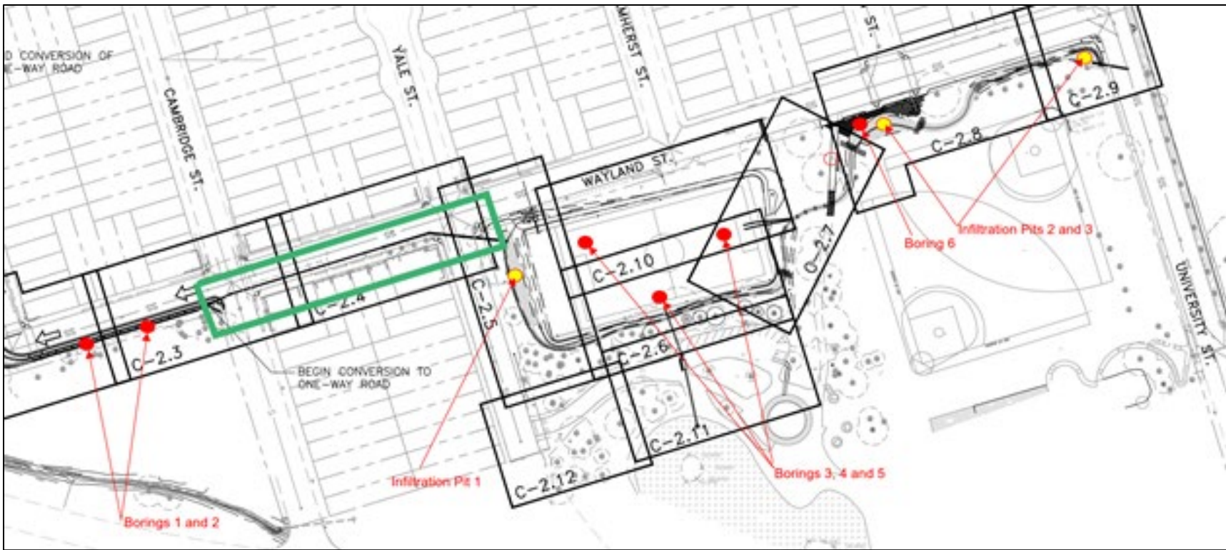
Figure 1. Proposed Geotechnical Investigation Sites
