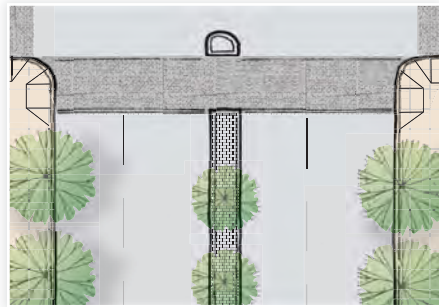
Pedestrian refuges provide space for pedestrians to wait on longer crossings and may include pedestrian amenities.
