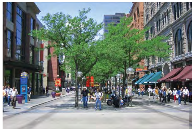
▲ The 16th Street Transit Mall in Denver provides standard sidewalks for pedestrians to walk along storefronts, dedicated lanes for transit vehicles, and a wide array of amenities and landscaping in the center of the right-of-way
