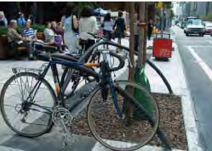
◀ Bike racks can be combined with other streetscape elements such as tree guards
