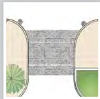
01 Raised crossing —at side access lanes (5.1)
