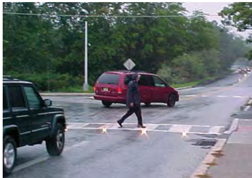
▶ In-roadway flashing lights enhance crosswalk visibility
