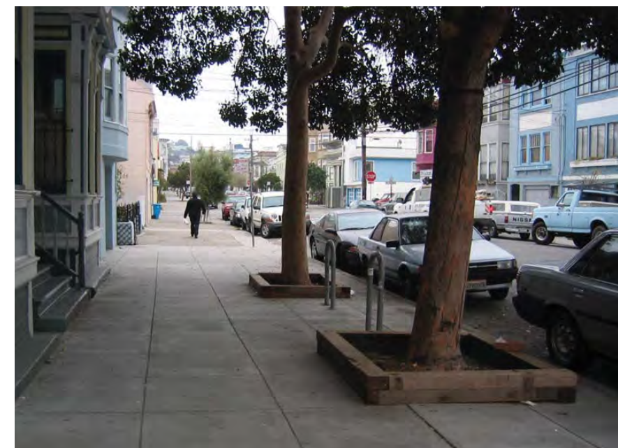
▼ Bike racks should be located near other streetscape elements, such as trees and planters, to cluster amenities
