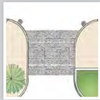
01 Rased crossing — at throughway intersections (5.1)
