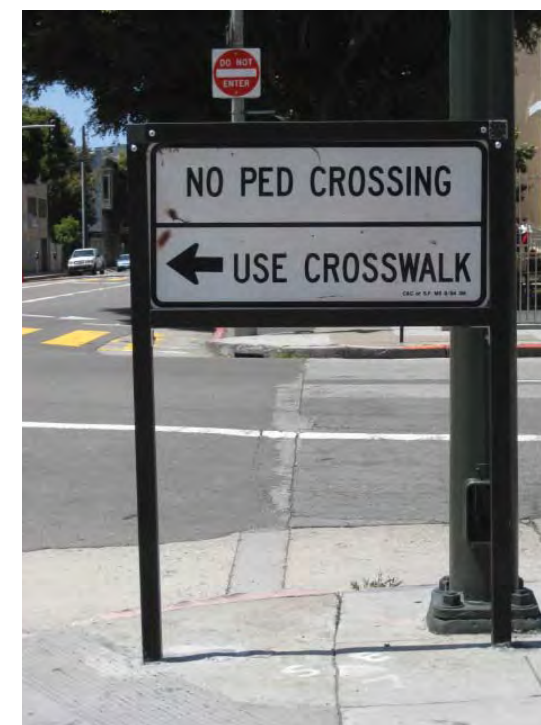
▲ Intersection leg closed to pedestrian crossing
