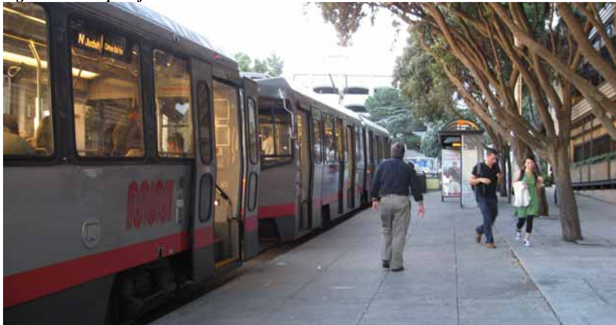
A 9' wide extension would allow customers to board the train directly from the sidewalk, similar to this bulb-out on Irving Street, between 2 nd Avenue and Arguello Boulevard.
