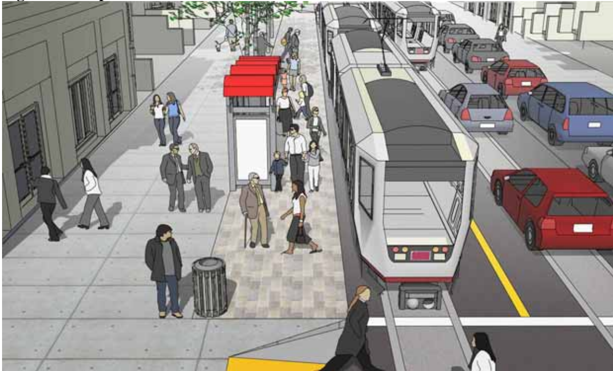
Rendering of proposed 9' bulb at Carl and Cole. Image courtesy of San Francisco Planning Department, City Design Group.
