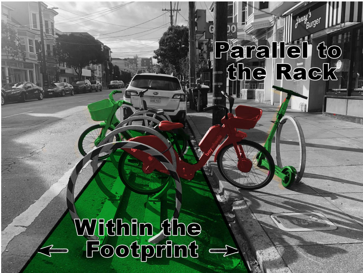
Figure 6 – Footprint of the Rack Illustration – The devices shaded in green depict devices parked within the footprint of the rack. The device shaded in red depicts a device parked outside of the footprint, which is considered improper. By parking outside of the rack footprint, devices impede the path of travel.
