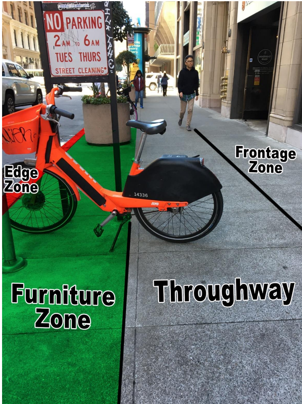
Figure 3 – Additional Furnishing Zone illustration – This device also extends outside of the furnishing zone, impeding the throughway.
