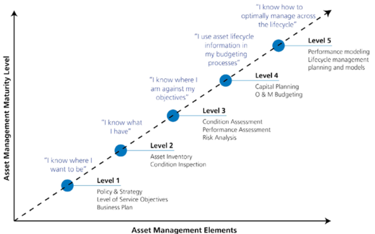
Figure 2: A Complete Performance Model (Includes asset life cycle management and capital planning)
