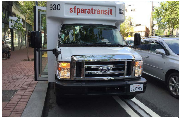
Paratransit vehicle "Perched" on Vertical Curb
