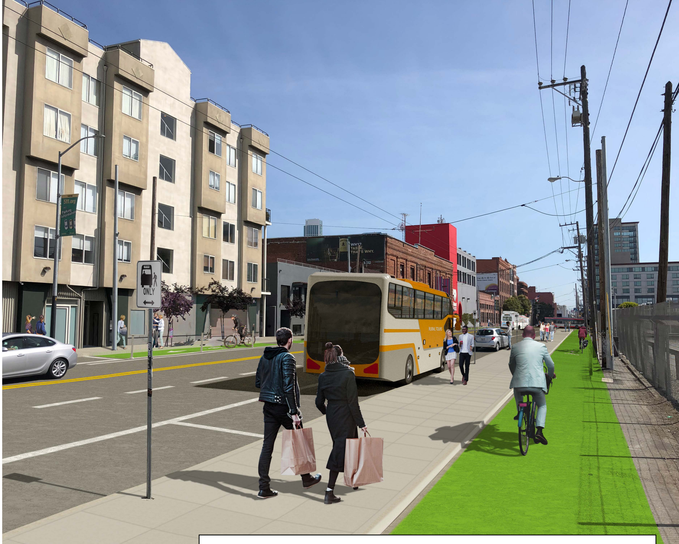
Bikeway adjacent to Caltrain property protected from moving traffic by floating walkway and boarding island
