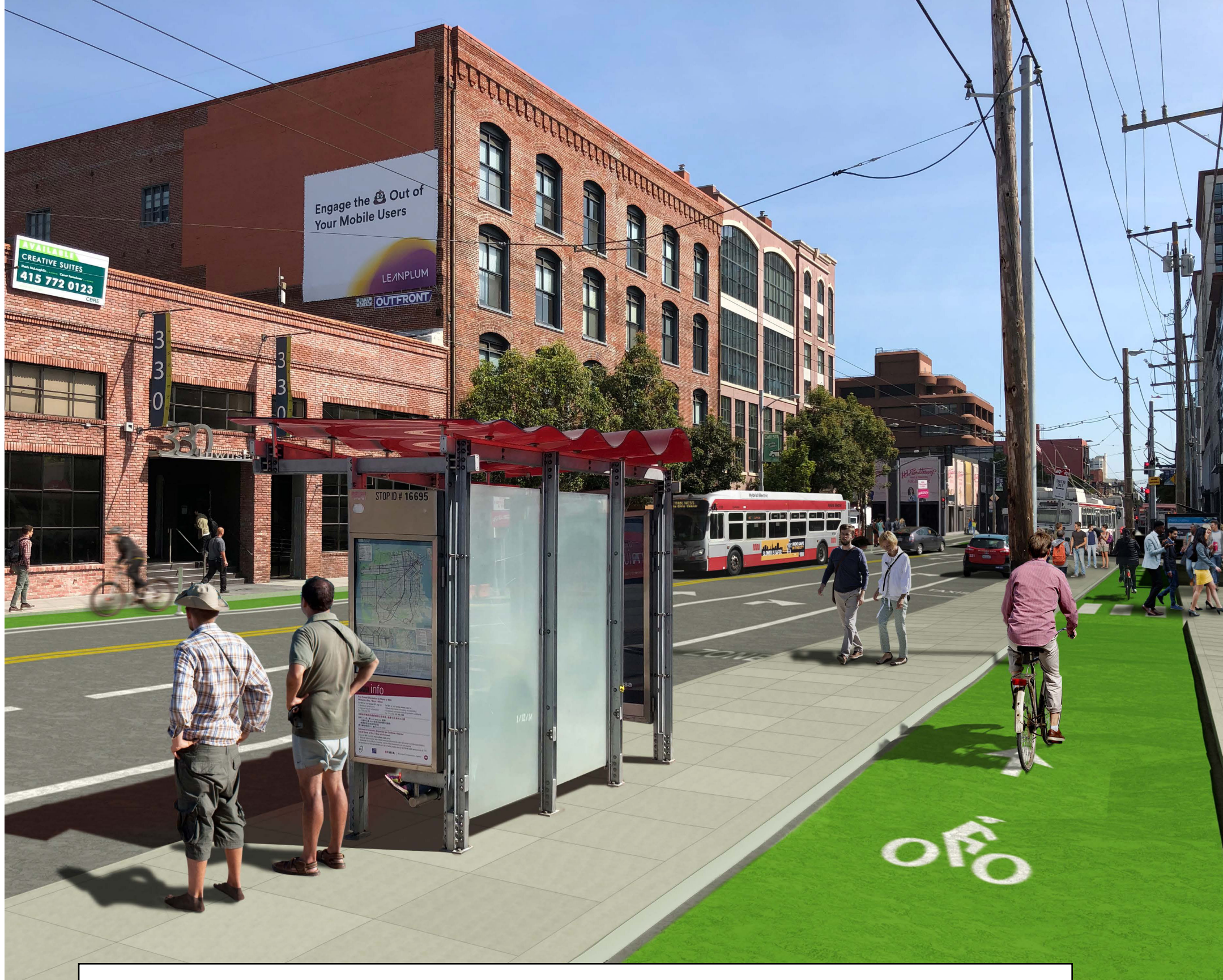
New floating walkway and boarding island for pickups and dropoffs by buses, taxis, TNC vehicles, shuttles, personal vehicles
