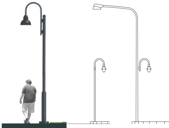
Figure 6.1 – New pedestrian-scale fixtures (left) and retrofitted existing fixtures (right).
