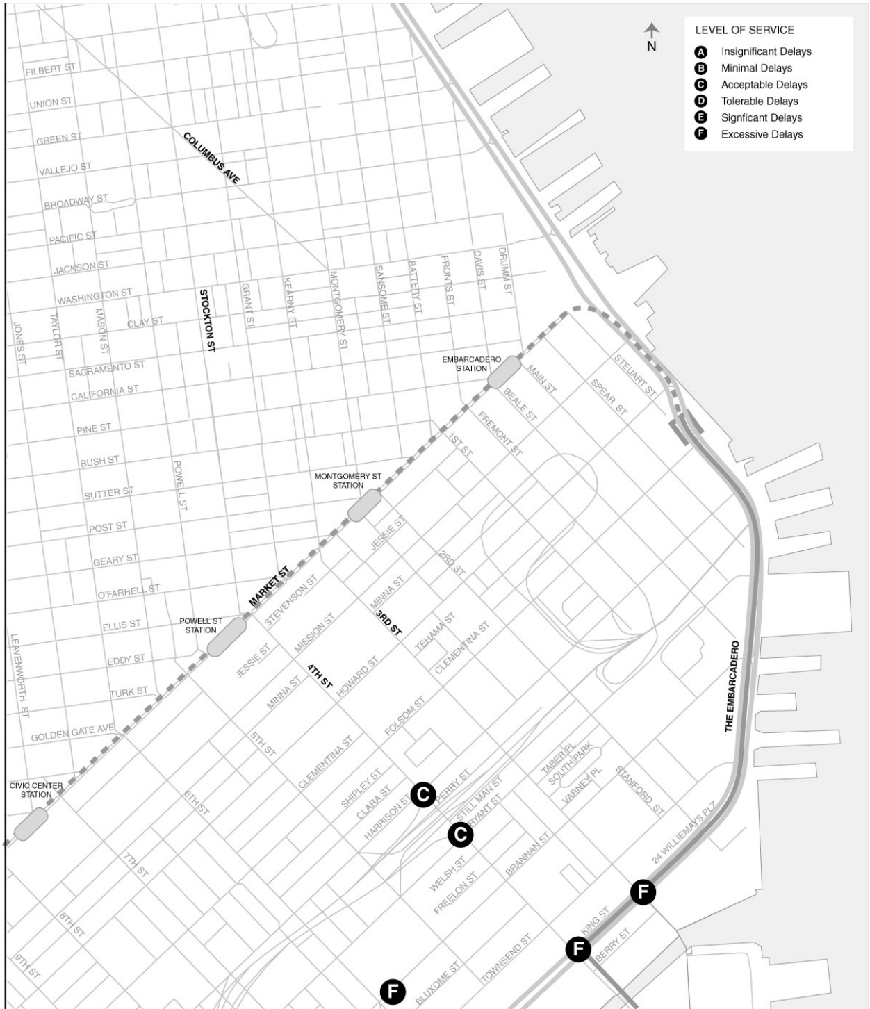
FIGURE 1-3 CENTRAL SUBWAY AND THIRD STREET CORRIDOR PROJECTED 2030 LEVEL OF SERVICE (LOS) AT VARIOUS LOCATIONS
