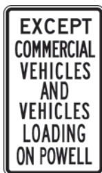
Image 2: Example of Vehicle Exemption Sign for motorists turning left from westbound Geary Street onto southbound Powell Street
