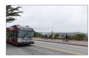
**Serving the Presidio:** Muni Forward extended the 30 Stockton to the Presidio using battery technology on new buses, without having to install new trolley wires.
