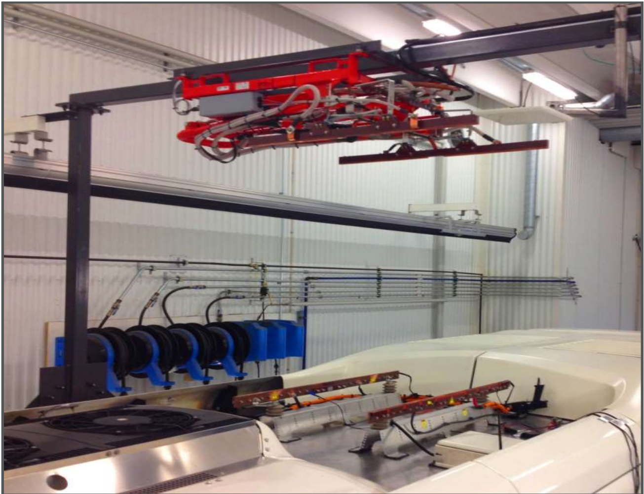
Figure 3-1. Inverted Pantograph and Charge Rails
