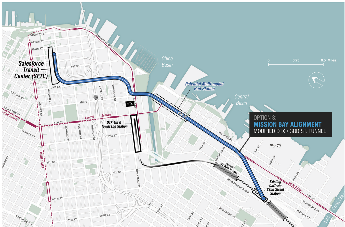
Exhibit 11: Mission Bay: Modified DTX + 3rd Street Tunnel Rail Alignment (Option 3)
