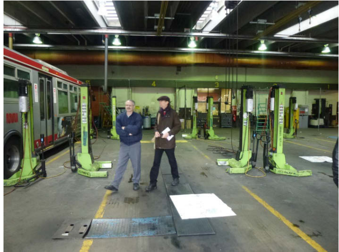
Portable Lifts in Maintenance Area
