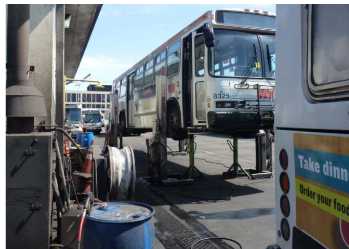
Portable Lifts and Pressure Wash Area
