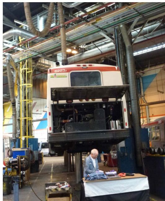
Vehicle Exhaust System Poorly Located
