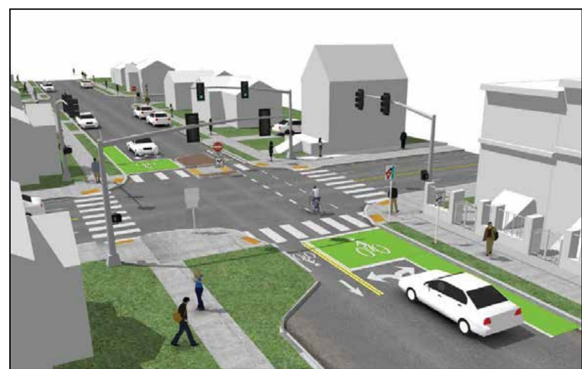
Rendering of a partial diverter at a neighborhood intersection. NOTE: see Diverter Details Board for further information.
