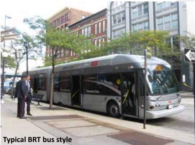
Multi-door boarding from platforms
