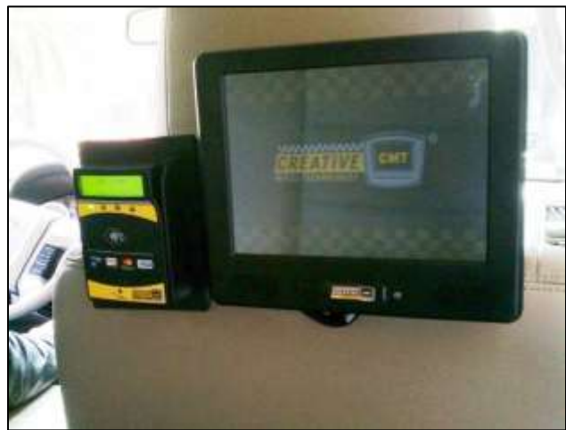
Passenger information monitor (PIM) & back seat credit card swipe used by Creative Mobile Technology (CMT)
