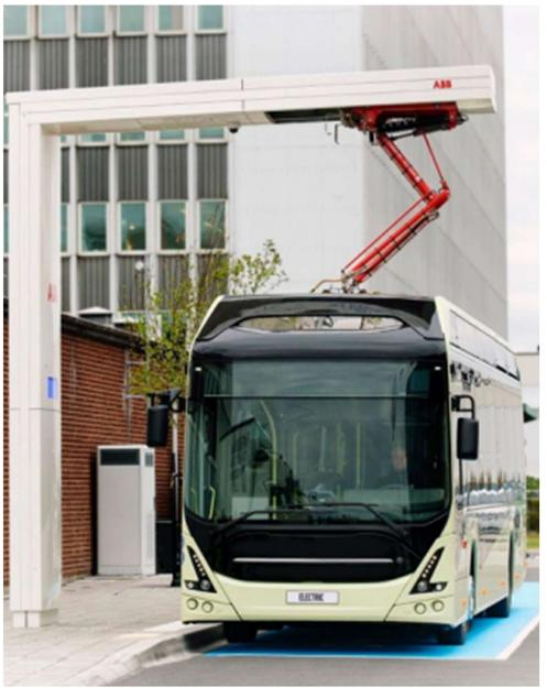
2022 SFMTA Rollout Plan, showing an ABB pantograph
