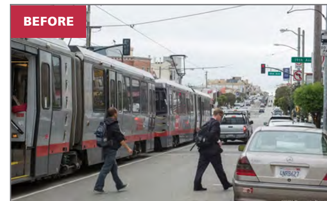
Boarding into a lane of traffic, before improvements: Before the project, passengers at most stops got on and off the train into an active traffic lane, leading to 24 injury collisions in five years.
