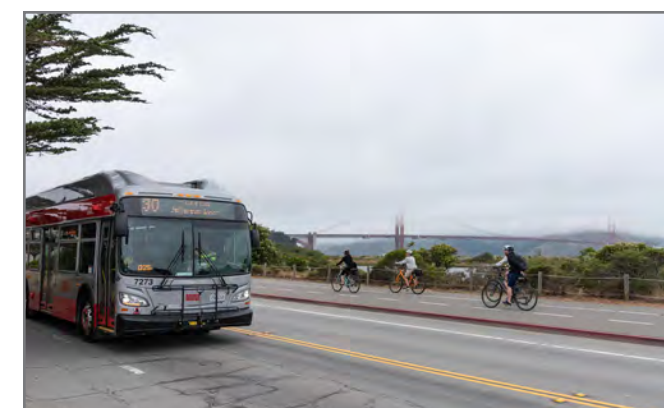
Serving the Presidio: Muni Forward extended the 30 Stockton to the Presidio using battery technology on new buses, without having to install new trolley wires.
