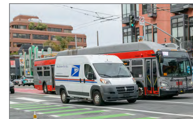
Queue jump at Townsend Street: A "queue jump," or short transit lane, on Townsend Street approaching 3rd Street helps the bus bypass traffic congestion where delays are most challenging.
