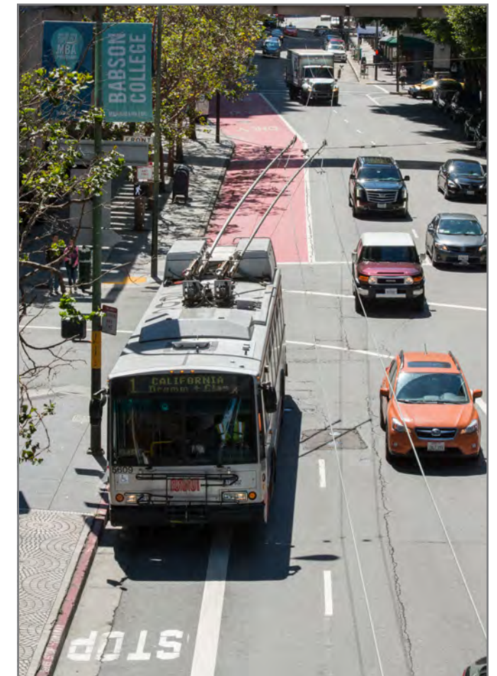
Clay Street red transit lane: A red transit lane on Clay Street helps to reduce delays for the 1 California in the Financial District.
