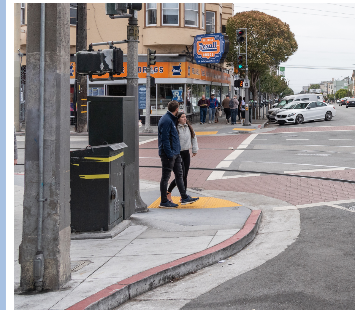
Install pedestrian bulbs (corner sidewalk extensions)
