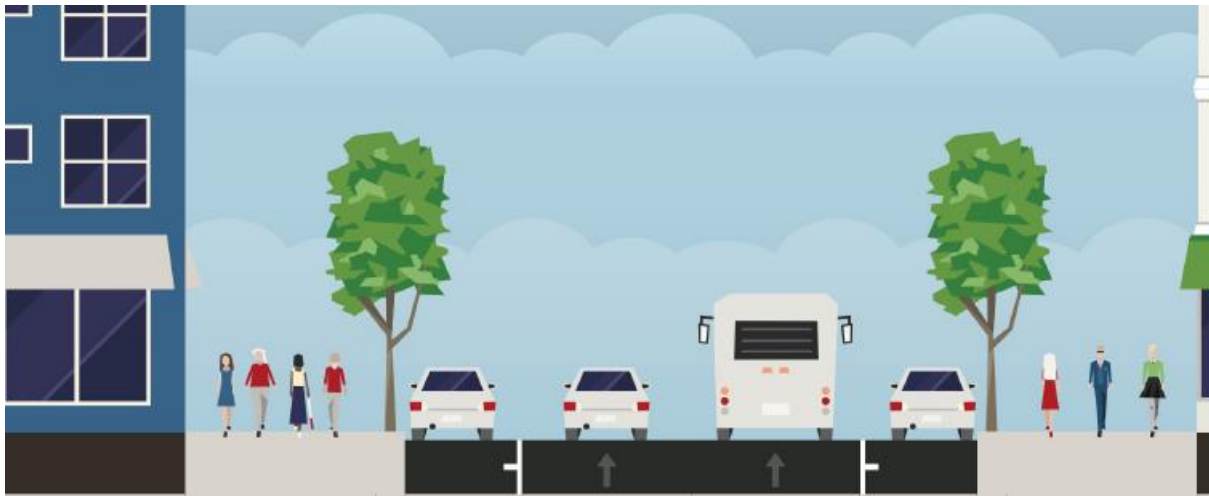
Figure 7 - Proposed cross-section: segments of Sacramento and Clay streets between Franklin and Larkin streets. The curbside travel lane would become a temporary emergency transit lane.
