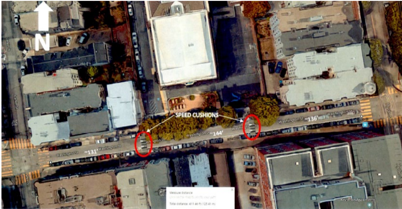
PROPOSED SPEED CUSHIONS ON WASHINGTON STREET BETWEEN LARKIN STREET AND HYDE STREET
