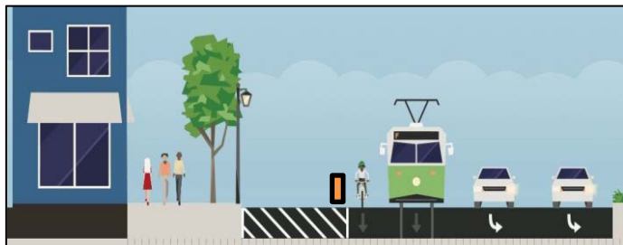
Construction zone (behind orange barrier) with temporary bike lane for working hours
