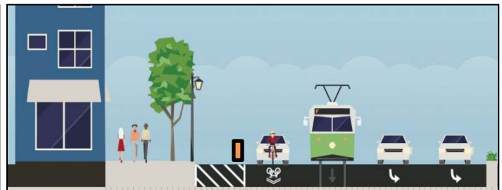
Construction zone (behind orange barrier) with shared lane for non-working hours
