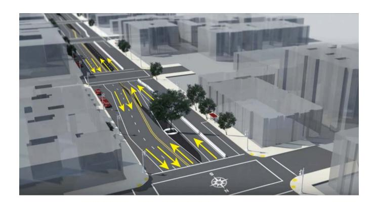
Pictured above: Screen shot from construction sequence animation illustrating two lanes traveling in the same direction separating as they pass on either side of median islands where one of 12 trees are protected for construction. Arrows added for emphasis.
