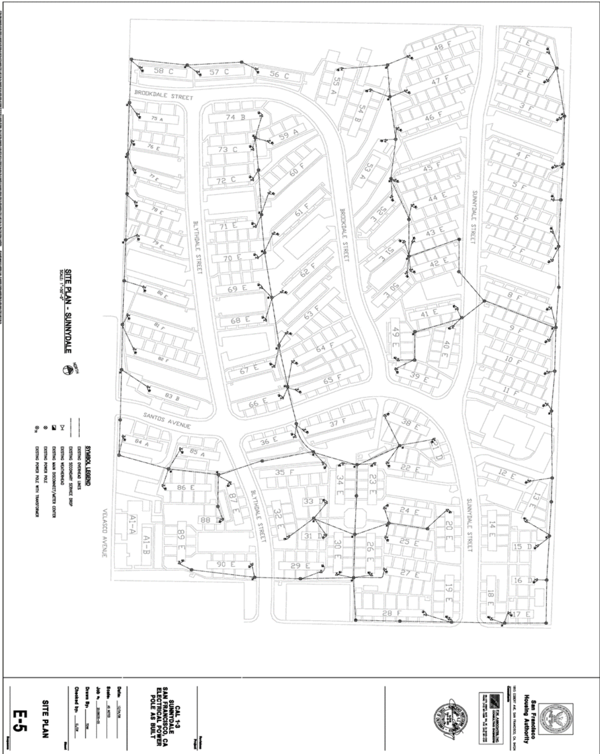
Figure 14.1 – Existing Electrical distribution at Project Site
