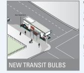
Wider sidewalks that "bulb" out at bus stops allow buses to board passengers without having to pull out and then back into congested traffic. They also provide space for shelters, signage, and other amenities.
