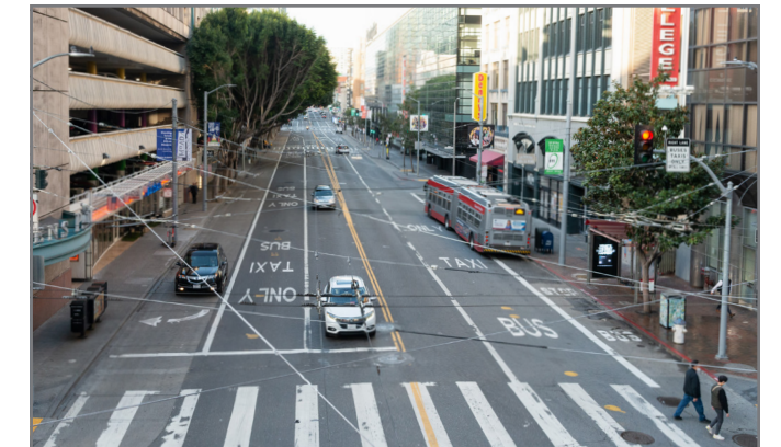
Temporary Emergency Transit Lane in SoMa: New 24/7 transit lanes were installed in SoMa in 2020, which were later approved to remain permanently and upgraded with red colorization.
