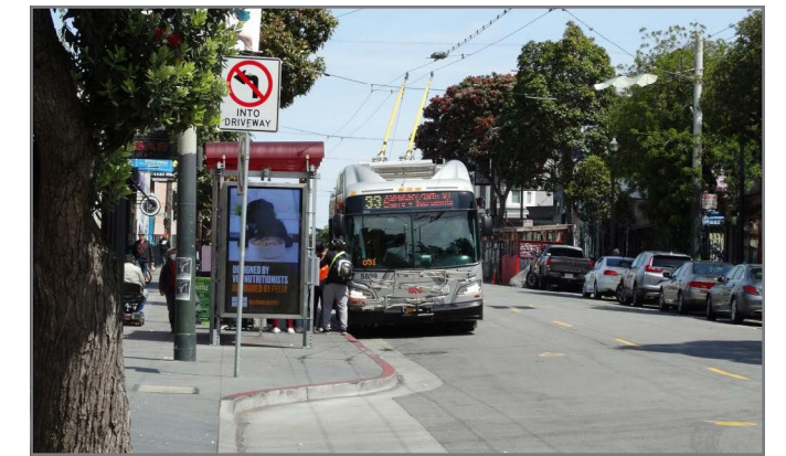
Wide boarding platforms on Haight Street: Transit bulbs on Haight Street, shown here at Stanyan Street, reduce boarding delays, improve safety and leave more space for stop amenities.
