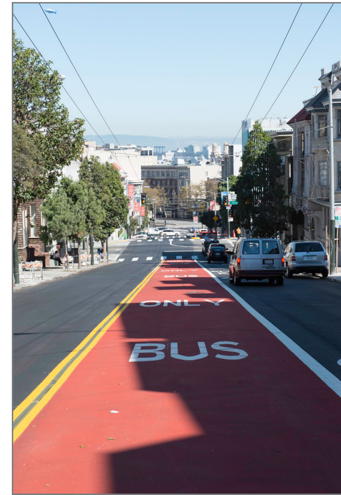
Haight Street red contraflow lane: A contraflow transit lane on Haight Street approaching Market Street makes bus trips more direct, avoiding a circuitous detour that added 2 minutes per trip.
