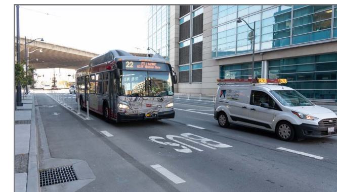
Extension to Mission Bay: Muni Forward extended the 22 Fillmore to Mission Bay, including a transit lane that is now colored red, providing direct access to UCSF and the Chase Center.
