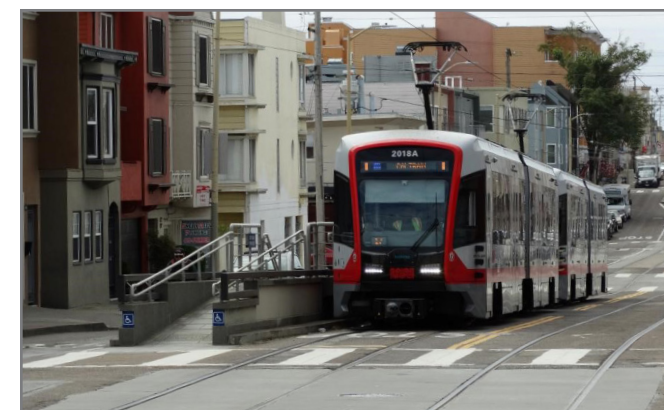
Wheelchair-accessible boarding platform (example 1 of 2): The wheelchair-accessible boarding island platform on Judah Street at 28th Avenue provides access to high-floor trains.
