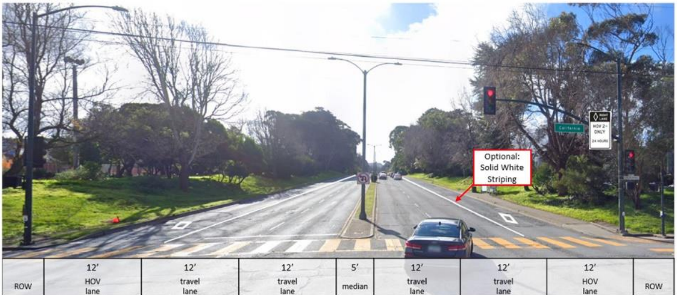
Figure 3: Cross Section Views of Existing and Proposed Conditions on Park Presidio at California
