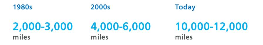
Mean Distance Between Failures (MDBF) is the industry-standard measurement of vehicle reliability. It tracks how long a vehicle travels before a mechanical failure that results in lost service.
