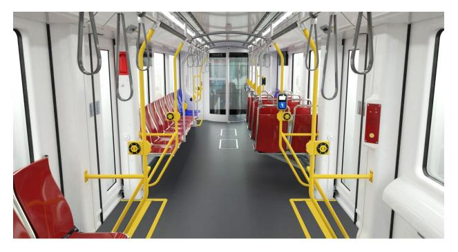
The carshell weight is expected to increase to accommodate structural reinforcements needed to handle the load of double-wide transverse passenger seats. The preliminary engineering work includes a carshell analysis to understand the structural changes necessary to support the new seating arrangement and verify that these changes can be accomplished within the 80,000-lb. weight limit of each vehicle.
