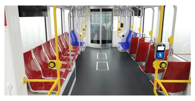
The final 101 Phase 2 vehicles (Nos. 2119-2219) will have a significant re-design to accommodate a new interior seating layout with double transverse seats as demonstrated in the rendering below and including:
