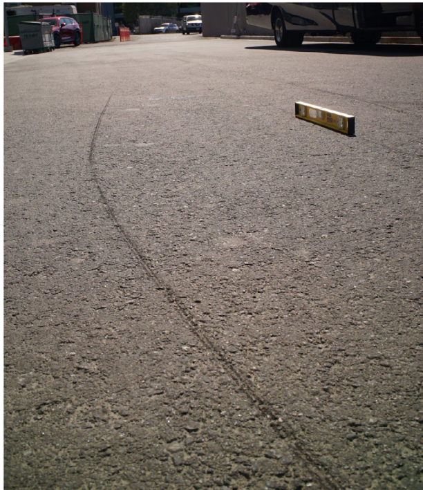
Image 4 (above): Wheel skid mark from field testing scooter on dry, level, clean pavement.
