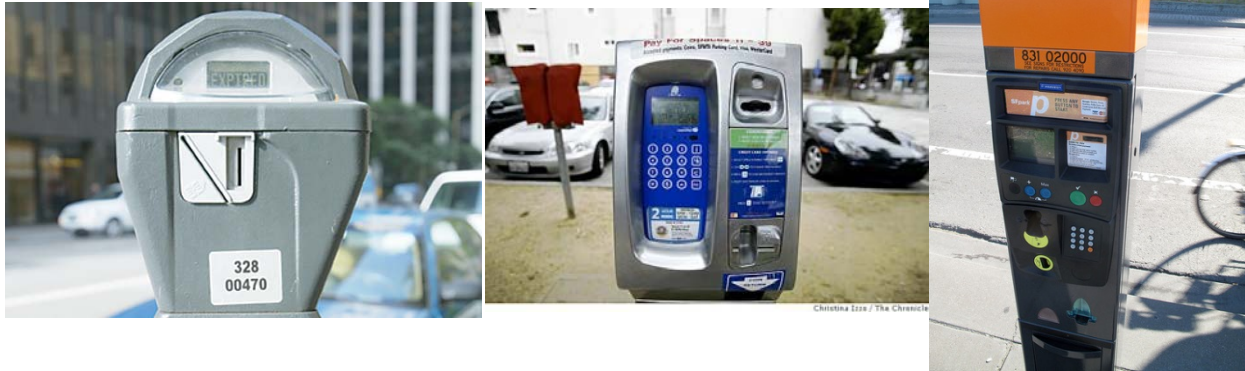
(Left) A MacKay single space meter. (Center) A Duncan RSV2/3 (Right) A Parkeon multi-space meter
