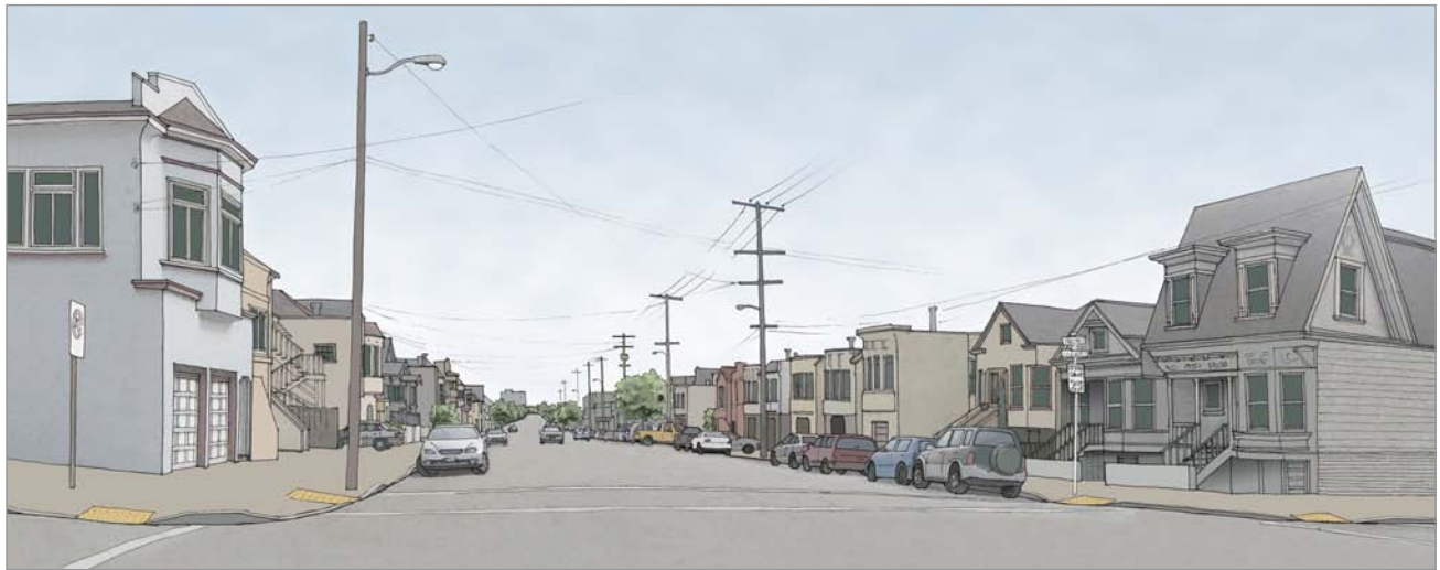
Figure 6-9. Alternative A-1: Perpendicular Parking on Alternating Sides (Sketch View)
