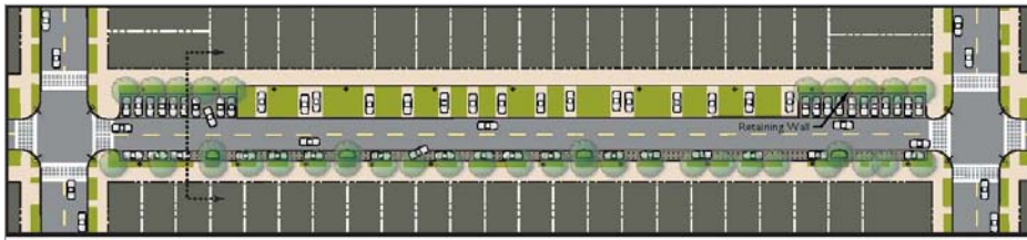
Figure 6-8. Alternative B, Perpendicular Parking in Hillside Areas: Plan View
