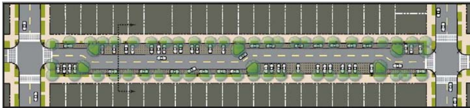
Figure 6-4. Alternative A-2, Perpendicular Parking on One Side: Plan View
