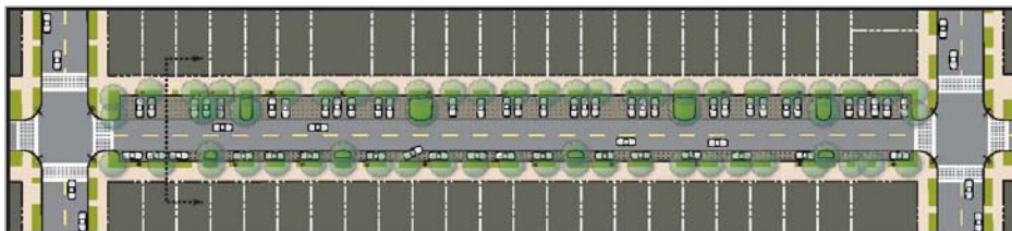
Figure 6-4. Alternative A-2, Perpendicular Parking on One Side: Plan View
