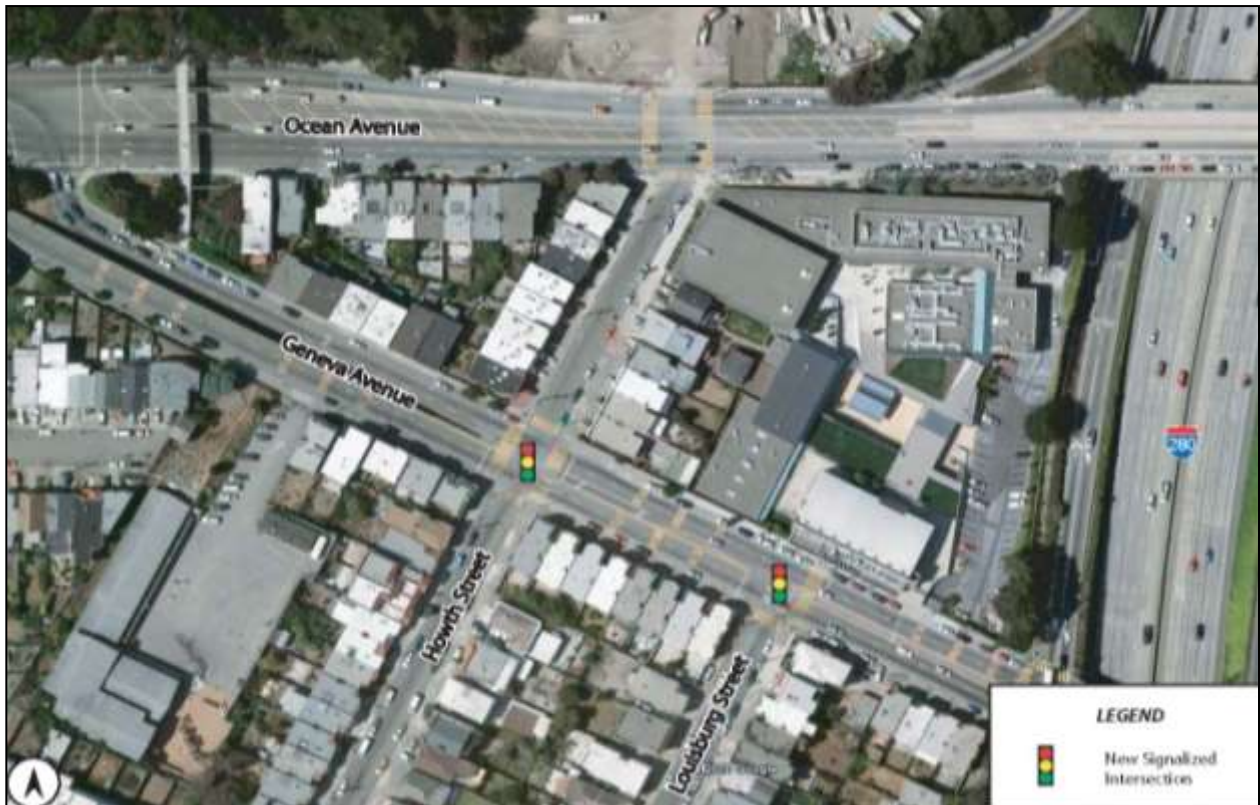
Figure 50: Improvement 21 - Signalization of Geneva Avenue and Howth Street and/or Geneva Avenue and Louisburg Street This map shows the location of the intersections of Geneva Avenue and Howth Street, as well as Geneva Avenue and Louisburg Street, both to the east of I-280 and south of Ocean Avenue.
