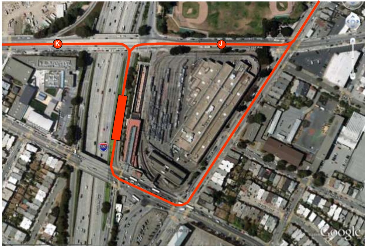
Figure 42: LRT Rail Loop The J line would go West on Ocean and turn into the stub, which lies between and parallel to the BART Station and I-280. From there, a track would go south in this right of way to Geneva, East on Geneva and North on San Jose.
