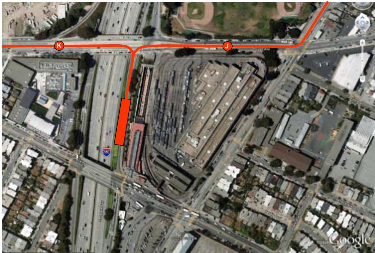
Figure 41: LRT Stub-End Station This map has an overlay which shows that the J would turn onto Ocean and go Westbound, and the K would be on Ocean. Both lines would turn on a track and into a stub which would lie between I-280 and the BART Station.
