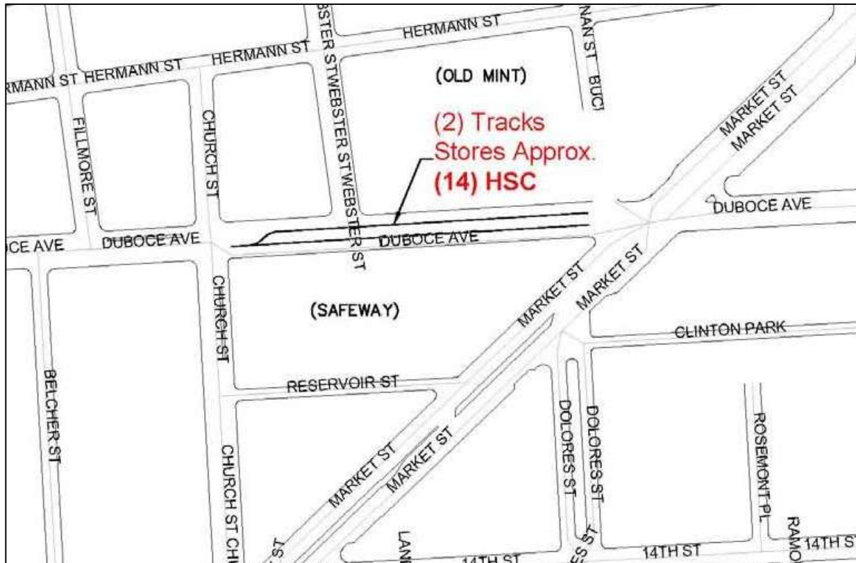
Figure 26: Duboce & Market Storage Tracks at Duboce Avenue and Market Street (Source: SFMTA) Figure demonstrates that the two tracks could accommodate 14 Historic Street Cars on Duboce Ave.
