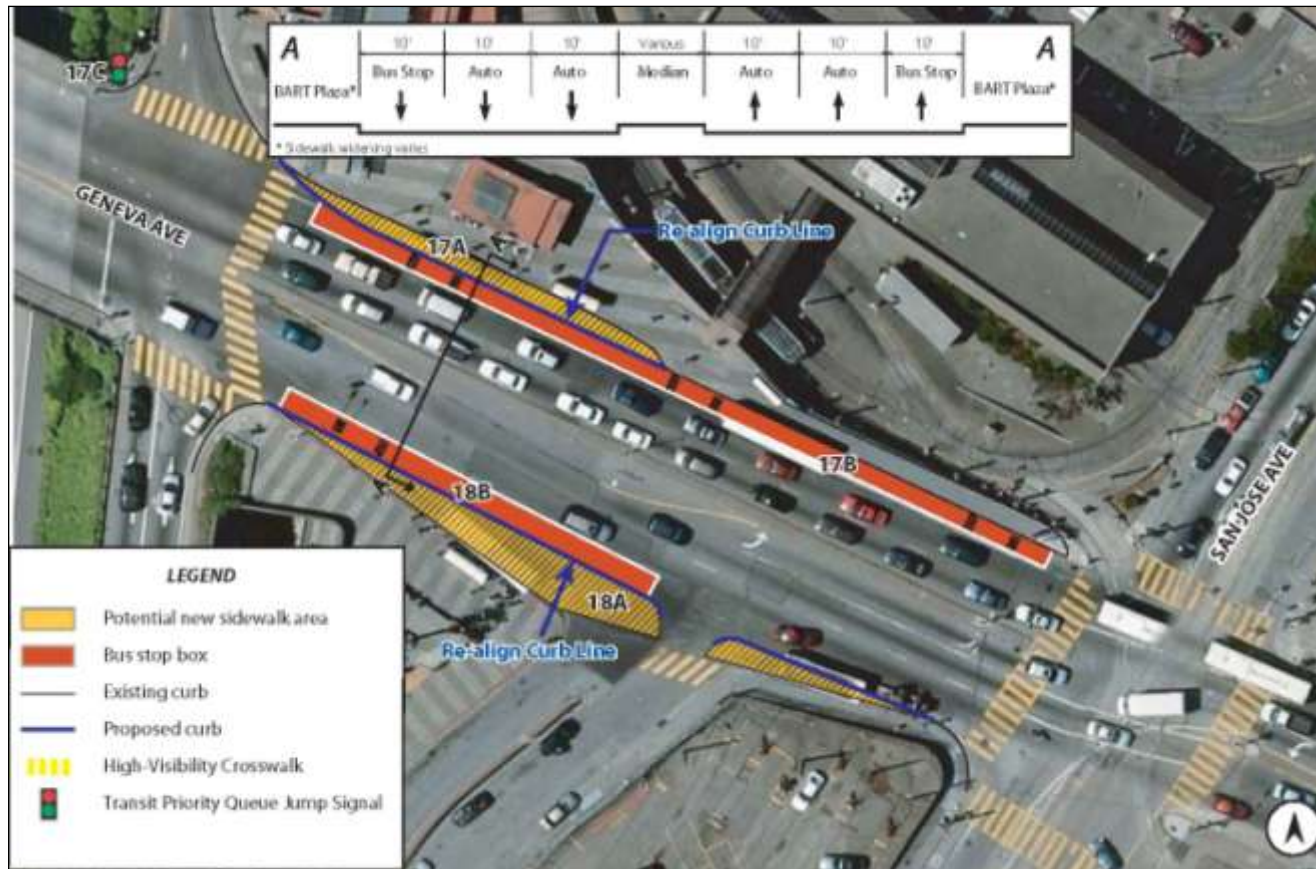
Figure 46: Improvements 17 and 18 - Westbound and Eastbound Improvements on Geneva Ave. This schematic shows a continental crosswalk at San Jose and Geneva Avenues. Also, there would be a continental crosswalk on the I-280 on and off ramps at Geneva, with a continental crosswalk across Geneva on the BART Station side. There is a proposed bus stop box on the north side of Geneva Avenue almost from the corner of San Jose Avenue to the I-280 on ramp, with an extended sidewalk for the western half. On the opposite side of Geneva Avenue, the sidewalk would be extended. There would be a bus stop box extending from the kiss-and-ride area to the I-280 off ramp.
