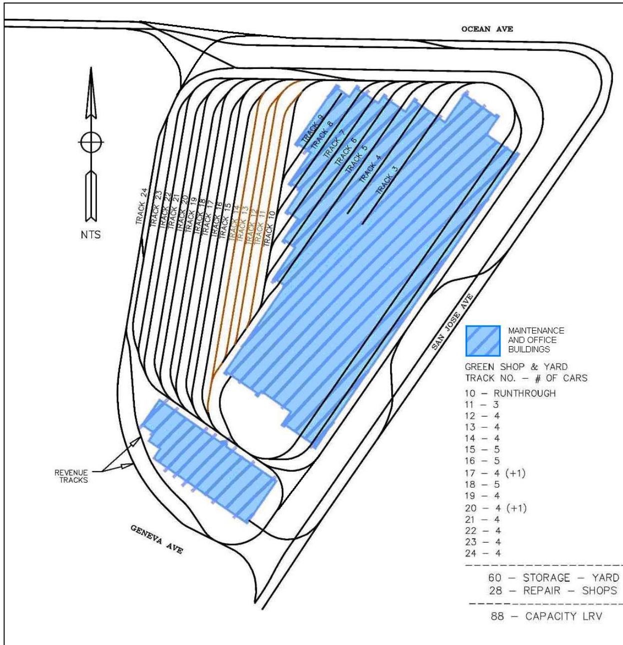
Figure 21: Green Yard Storage and Maintenance Facility (Source: SFMTA)
