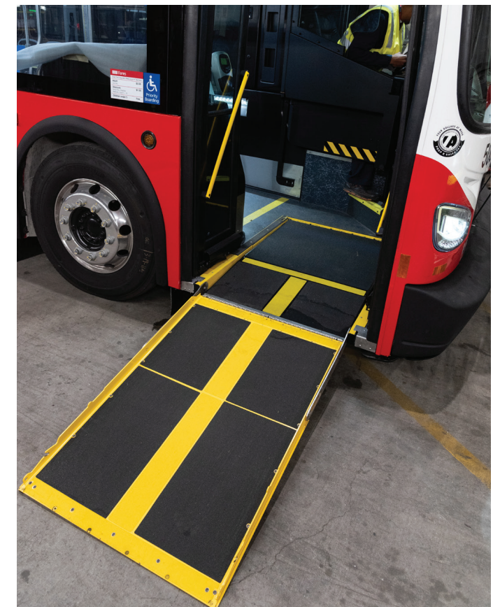
Figure 1-5: Upgraded Wheelchair Ramp
