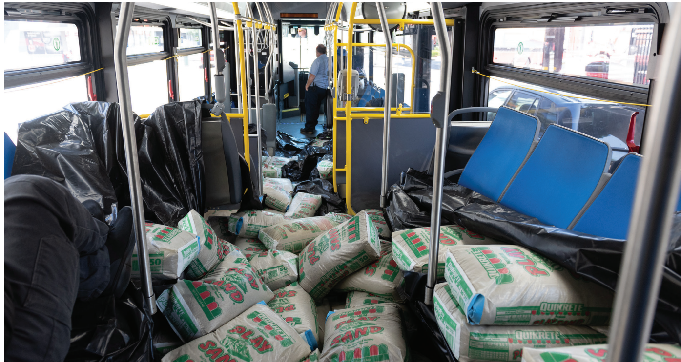
Figure 6-6: Loaded Bus During Testing
