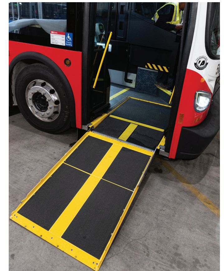
Figure 1-5: Upgraded Wheelchair Ramp
