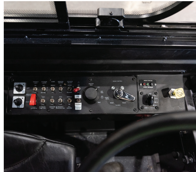
Figure 7-2: BYD bus 5004 Operator Side Panel Controls
