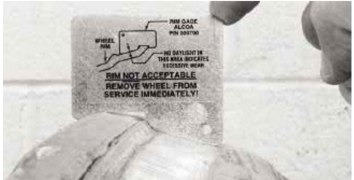
Figure 3-29: Not serviceable (scrap wheel)
