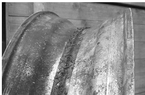
Figure 3-2: Discoloration of Wheel with charred rubber
