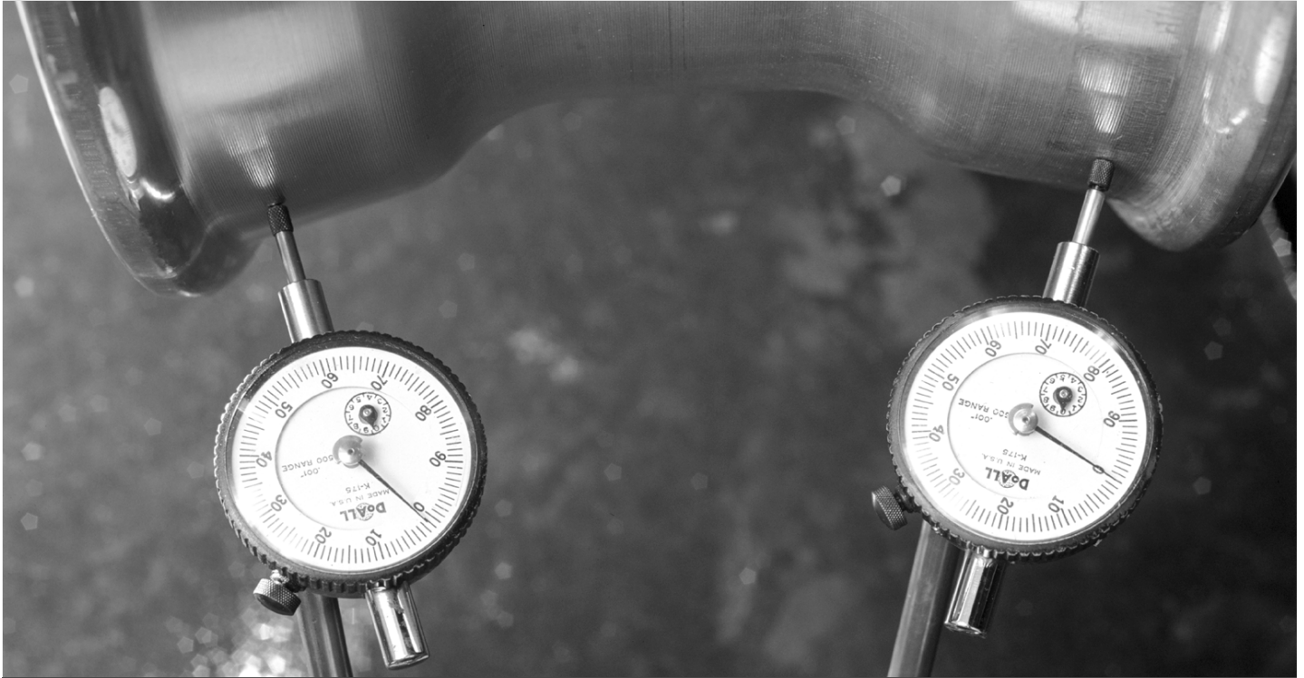
Figure 3-10: Inspect tire mounting according to instructions.
