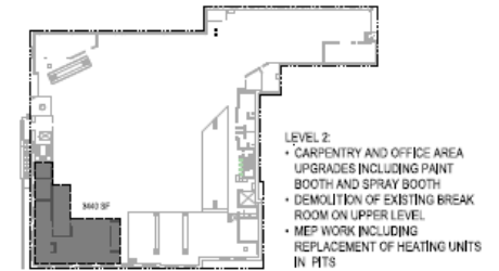
3B PHASE 3B | CARPENTRY UPGRADES 1" = 40'
