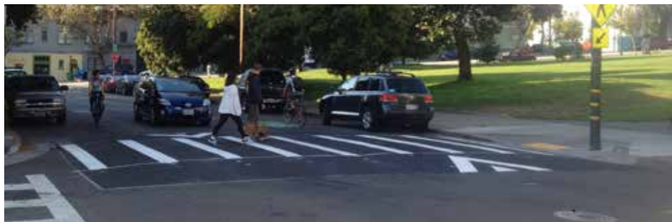
Raised Crosswalk with High-visibility Markings
