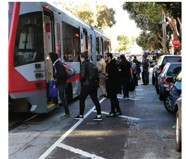
Buffer Zone striping for traffic safety
