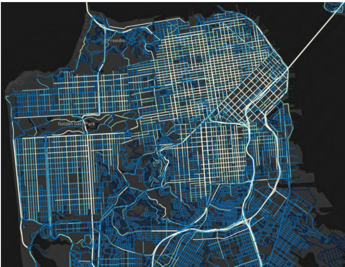
Mapbox measures human and vehicular activity in every city in America. This image shows probe density across San Francisco, where brighter is better: over 200 miles of road in San Francisco have data densities that allow extremely detailed, minute-by-minute analysis.
