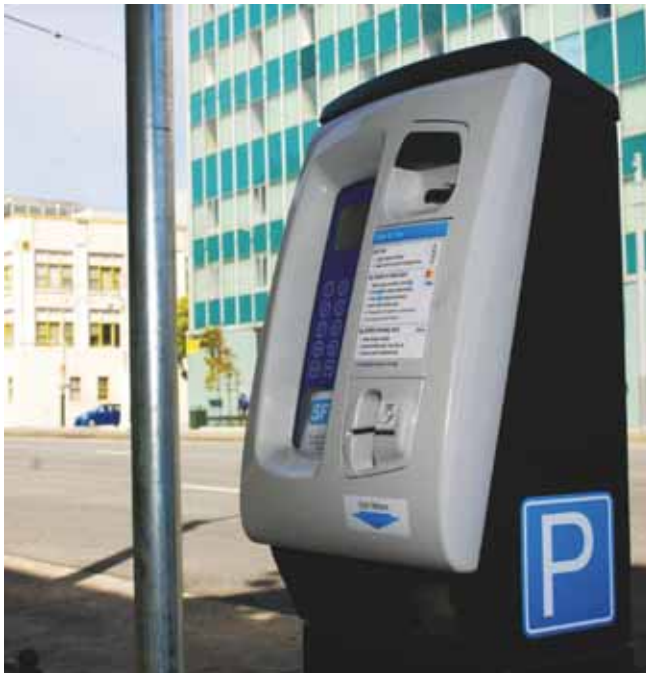
Image: Picture is of a parking meter which takes various forms of payment and variable pricing.
