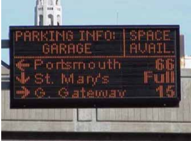
Image: Photograph shows the direction to three garages and how many spaces are available.
