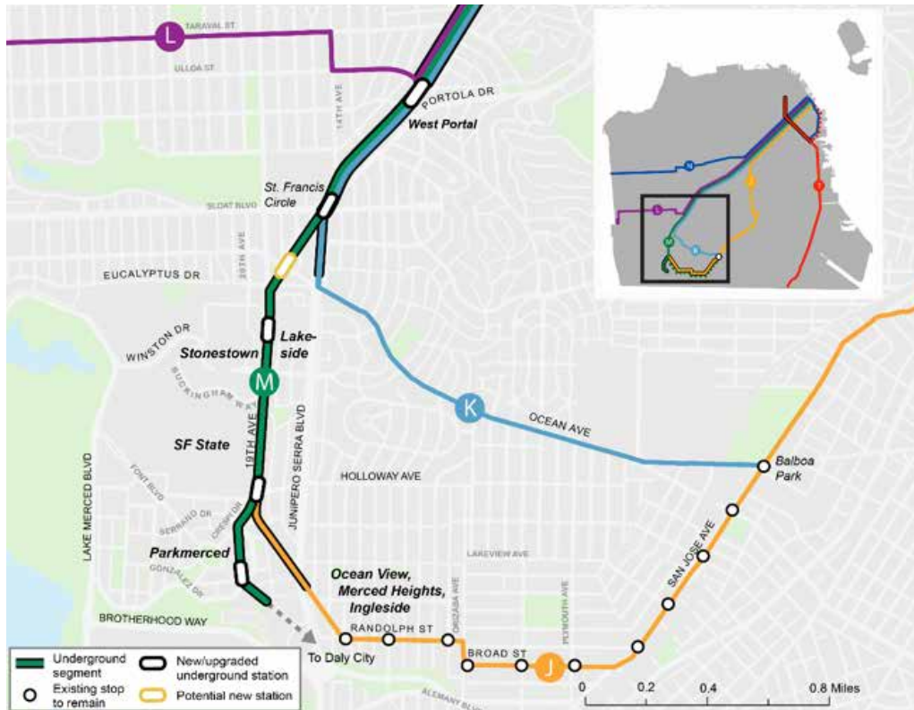
Figure 22. Subway Expansion Project Area
