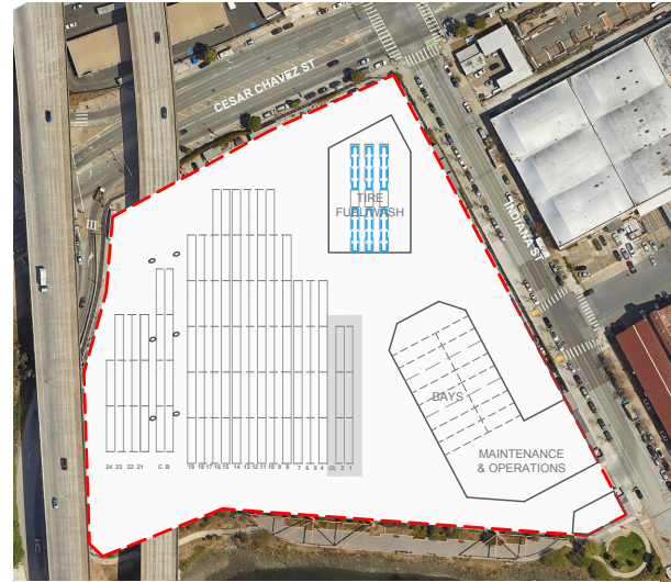
PILOT (lanes 1-3, shown in gray, closed during construction)
