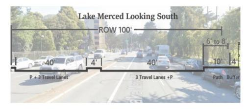
The existing roadway here is characterized by three southbound vehicle travels lanes and southbound one parking lane and three northbound vehicle travel lanes and one northbound parking lane. There is narrow path/landscaped area on the lakeside of the roadway and either a concrete median or striped median between southbound and northbound vehicle travel lanes. See cross section above for general roadway measurements.
