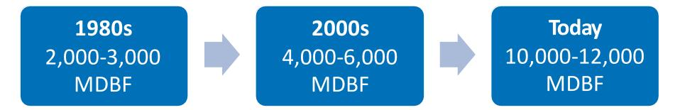
Mean Distance Between Failures (MDBF) is the industry-standard measurement of vehicle reliability. MDBF tracks how long a vehicle travels before an in-service failure
