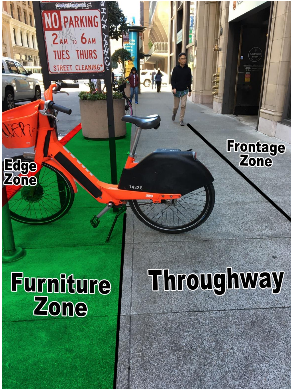
Figure 3 – Additional Furnishing Zone illustration – This device also extends outside of the furnishing zone, impeding the thoroughway.
