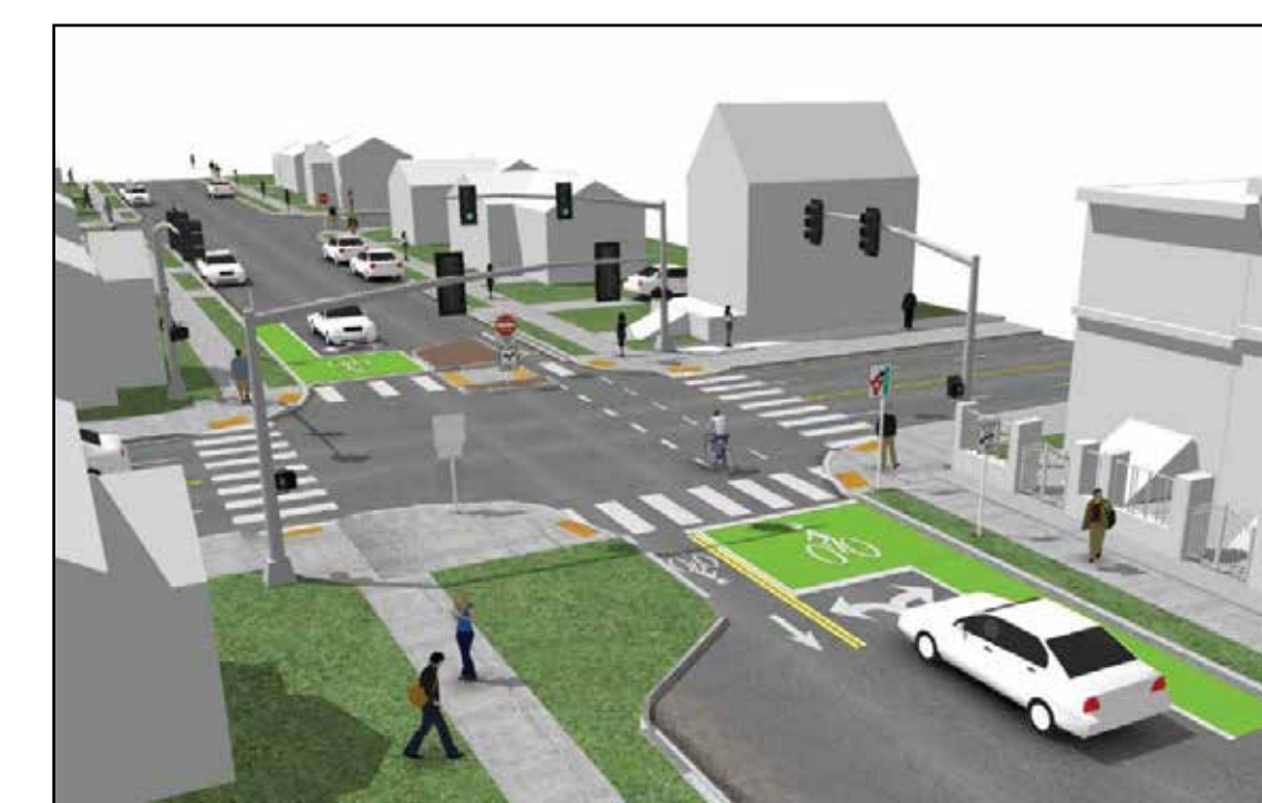
Rendering of a partial diverter at a neighborhood intersection. NOTE: all streets remain two-way, all driveway access would be maintained.
